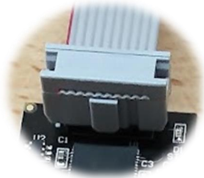
Figure 1: Programmer JTAG Connection
