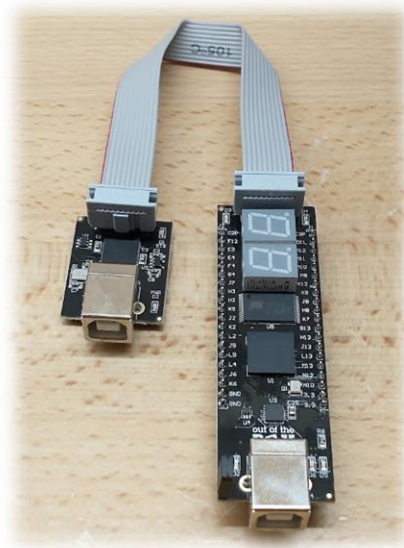
Figure 3: JTAG Cable Orientation
