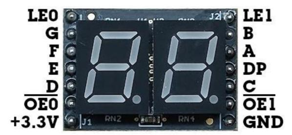
Figure 2: Breakout Board Pinout
